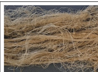
(a) Hemp extracted fibres at the Output of FRD line
