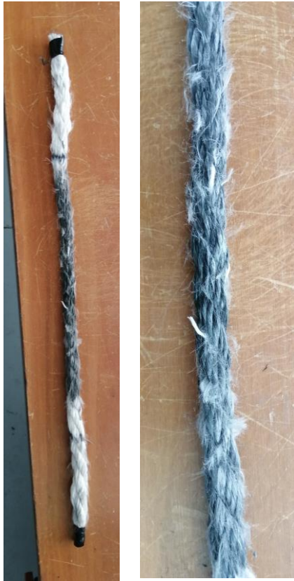
Sample after 29 %MBL fatigue test
